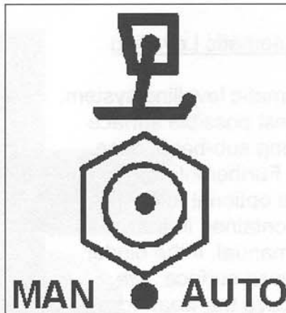
Toggle Switch S18 Operating mode of the levelling system MAN / O / AUTO
