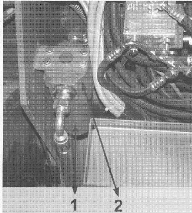
Pressure valve in the auger circuit
